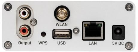
The WPS button for an easy connection with Wi-Fi routers and the port for the low-noise "medical grade" power adapter can be found on the rear of the Limetree Network
